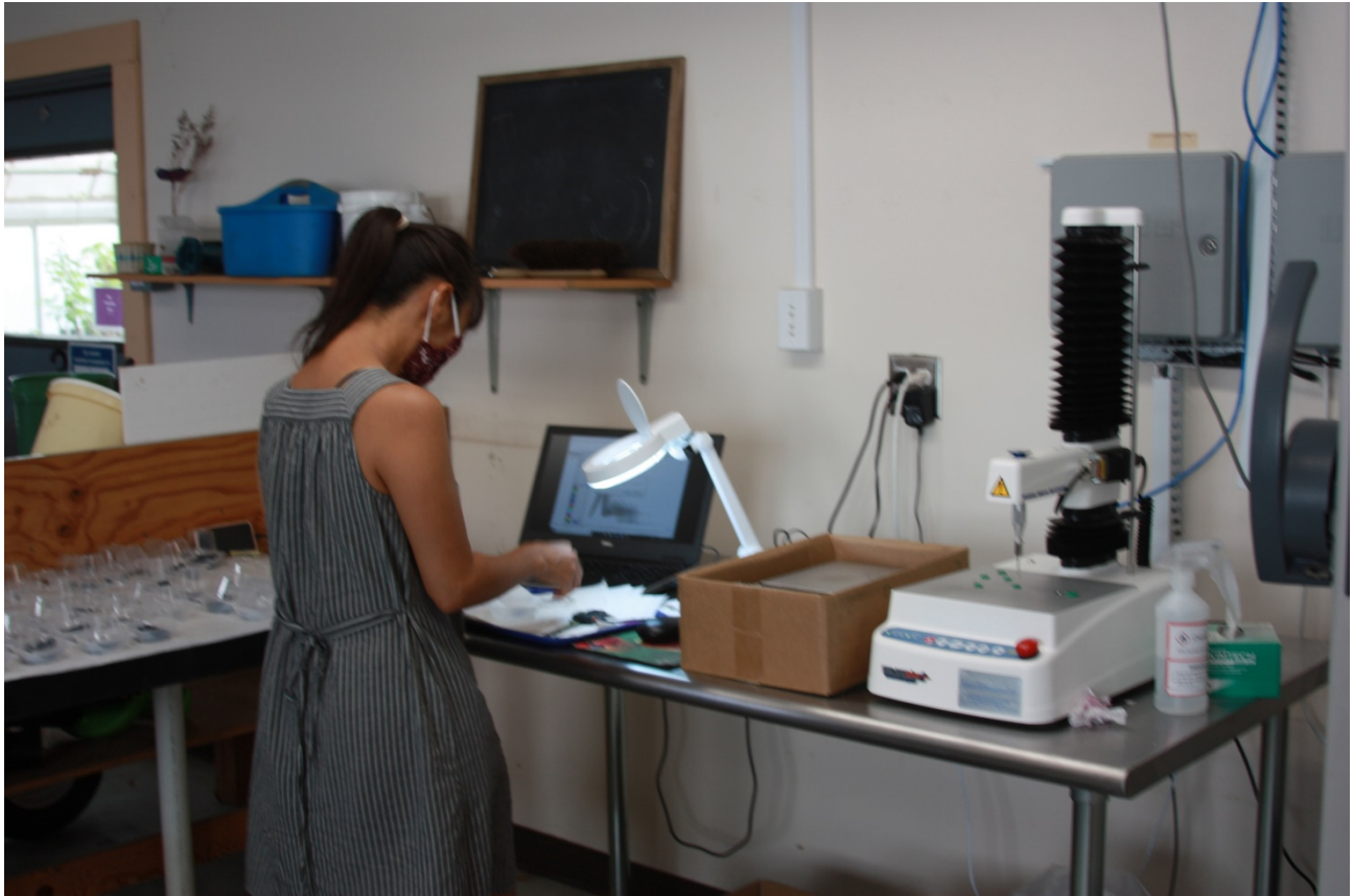
Postdoc Marti Pottorff (NCSU) using the Texture Analyzer to evaluate fruit characteristics and shelf life indicators in harvested ripe blueberry fruit.
